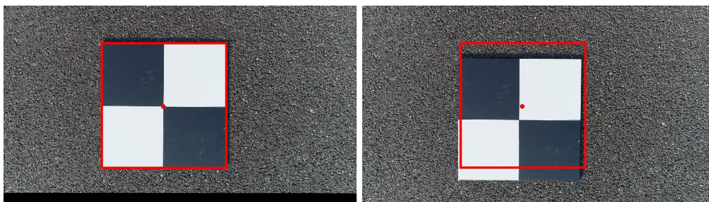
■ Figure 2 Registered image (left) and the raw drone image (right) of a Ground Control Point (GCP) from 1.5 m height. The borders of the left image are clipped due to translation and rotation. The red box depicts the GCP location at the first video frame, which was shot around 30 s beforehand.
